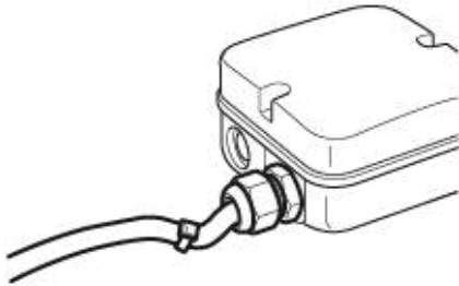
Fig. 2: Fan installed lying flat, cable routed in a U-shaped loop.
