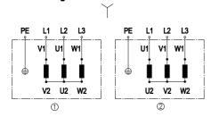
Change of rotation direction by reversing two phases
