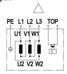
Note: Change of rotation direction by reversing two phases
