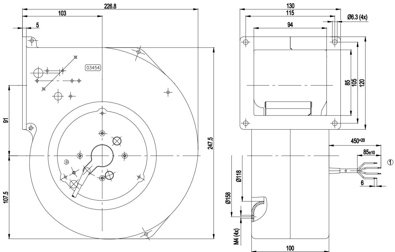
1 Connection line PVC 4G 0.5 mm<sup>2</sup>, 4 x brass lead tips crimped
