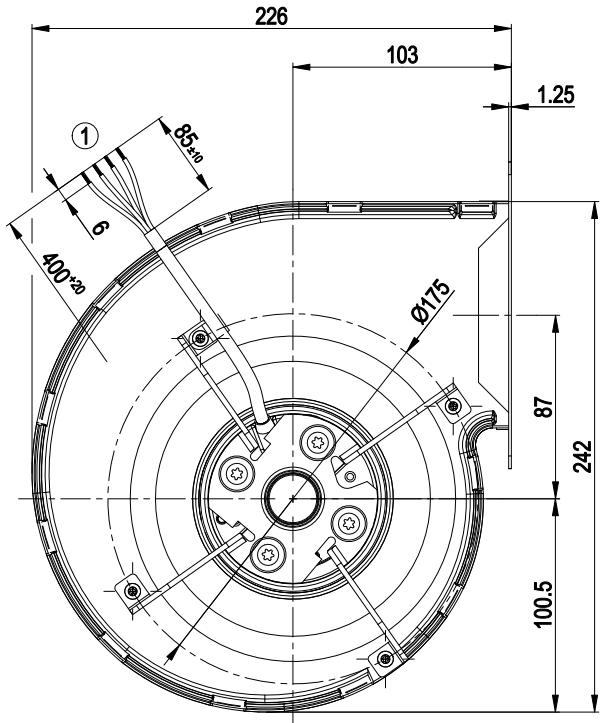
1 Connection line PVC 4G 0.5mm<sup>2</sup>, 4x brass lead tips crimped
